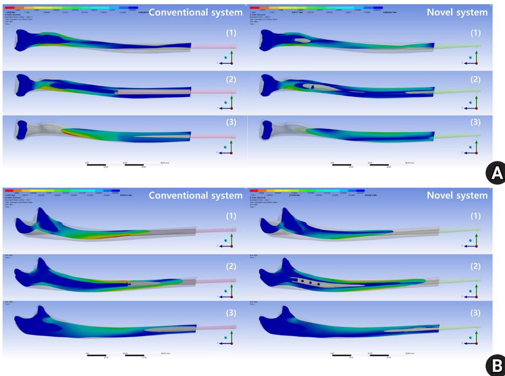
Fig. 5. Stress-distribution pattern when stress was loaded along the Z-axis at the radius (A) and the ulna (B).
